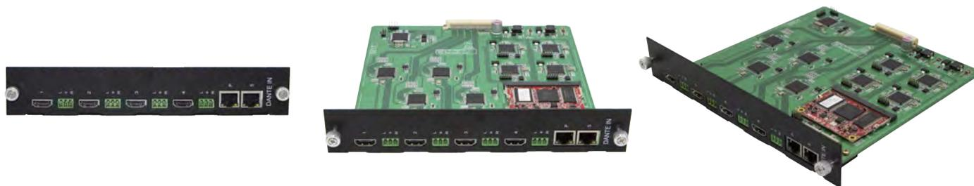
The **PM-HIS4-DA-U** is a Dante Audio with HDMI ports input board for PureMedia™ matrix switchers supporting UltraHD/4K resolutions and Dante/AES67 IP audio. Each **PM-HIS4-DA-U** has primary and secondary RJ-45 ports for IP audio, four HDMI ports, and four stereo unbalanced analog ports.
